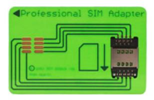
The professional SIM adapter is a great solution for temporarily converting a SIM-sized card to a full size one, allowing it to be used with a standard smartcard reader. The adapter has the same kind of locking connector as a mobile phone, linked via PCB tracks to solder-plated pads which come into contact with the reader. This adapter is a simple solution for regular SIM phonebook editing or for management of SIM-sized cards used for PC logon and security applications.
